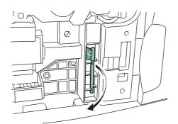
3 Pull up the lock lever on the left side of the printer, and open the left cover 1.
